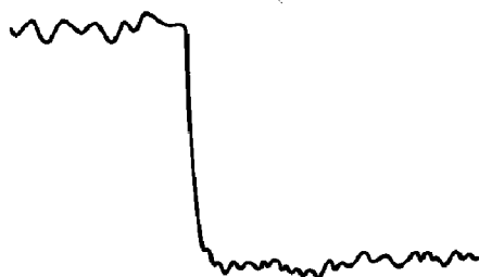
Fig. 1. Plot of light intensity at 250 nm vs. time after the flash in the 302.5 nm photolysis of a mixture of \text{C}_2\text{H}_5\text{CHO} at 15.0 Torr and air at 303.3 Torr. The time scale runs from left to right with a sweep time of 2 \mu\text{s} per channel. The total time of the trace is about 500 \mu\text{s} . The fraction of light absorbed is 0.012. The plot is an average of eight shots.
